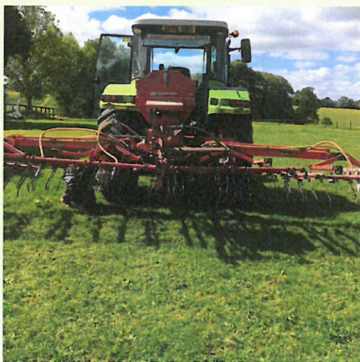
Adapted grass harrow will be used to establish grass on each site
