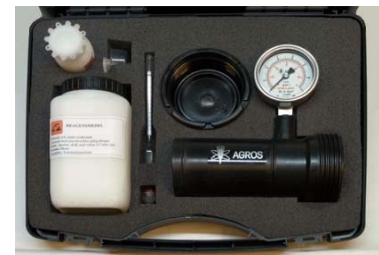
Agros on farm Nitrogen meter, including hydrometer to estimate Phosphate and Potash levels.
