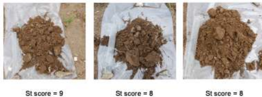
Figure 3-2 Examples of visual soil structure (ST) scores taken in spring 2013 at Norfolk (Defra project WQ0140) from conventional (plough-based) cultivation. The highest score (10) is given to the least compact and most porous condition, and the lowest score (1) to a massive condition with no structure and few or no cracks.
